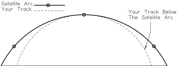
Adjustment Needed: Increase Motor Latitude. Decrease Declination. Move the Rotational Axis of the Dish Away From Horizontal.
