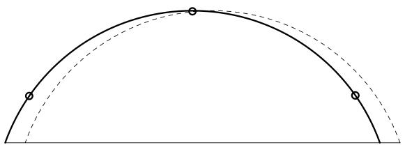
If your North/South Alignment is off, you will be Above the Arc on one side and below the Arc on the other side. Turn entire Polar Mount Assembly on the mast to correct.
