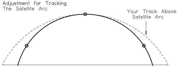
Adjustment Needed: Decrease Motor Latitude. Increase Declination. Move the Rotational Axis of the Dish Towards Horizontal.
